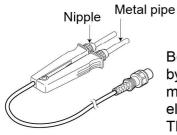
Before installing the tips, please loose the nipples by turning them counterclockwise and remove the metal pipes which are to protect the heating elements from damage during transportation. Then, insert the tips refering to the page 5 "Replacing the Tip/Tip selection" of the instruction manual.
